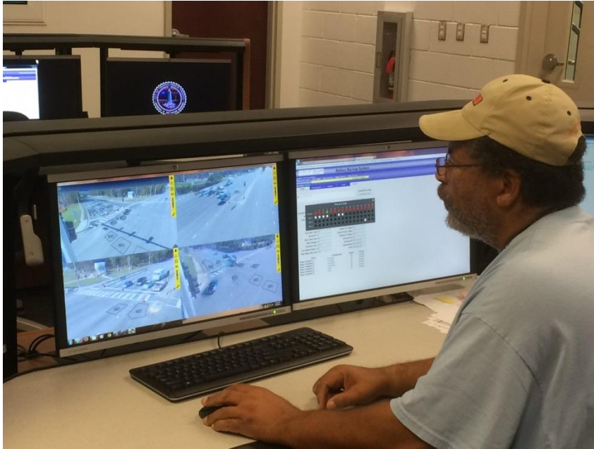
Staff member (Steve Smith) setting up vehicle detection and object masking zones
