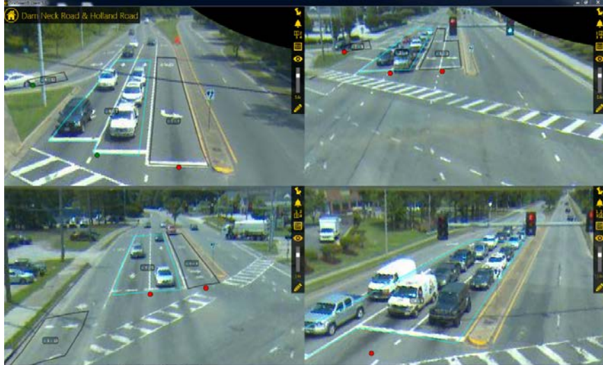
Quad view of the intersection - A fish eye view available - All views captured from 1 camera
