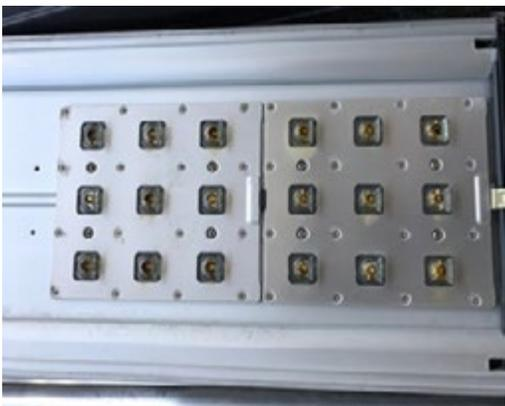
Damaged/Overheated LED Panels
