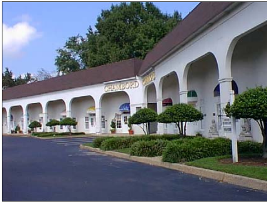
A good Maintenance plan and this Landscape design provide for Natural Surveillance opportunity in this strip shopping center, also allowing citizens in their normal activities to observe the space around them. Plant selection, it’s location, and it’s growth rate/maturation is important to consider when designing a space. The wrong tree or shrub can have an adverse affect on surveillance opportunities by users.
