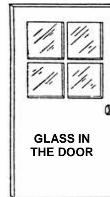
Doors containing windows or with adjacent glass panels can be easily defeated by breaking out a pane of glass, reaching in and unlocking the door.
