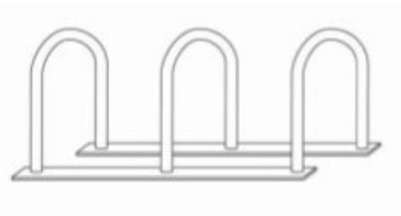
*Left: A simple plaza rack like this one that does not require drilling provides secure parking for 6 bicycles without damaging expensive paving materials. Graphic from Las Cruces Proposed Bicycle Parking Design Standards.*
