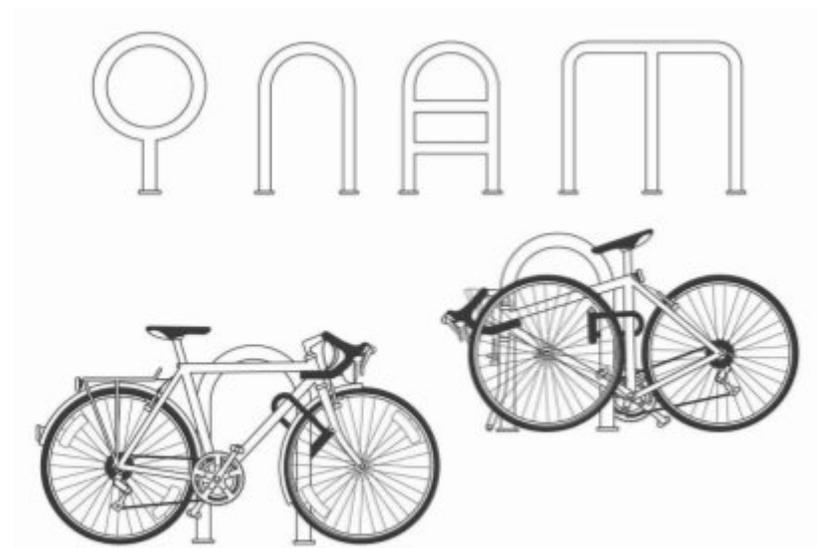
*Left: Examples of acceptable two-point support designs. Graphic from Las Cruces Proposed Bicycle Parking Design Standards.*
