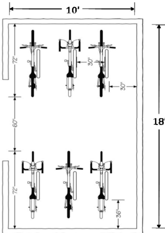
*Left: A 10'x18' vehicular parking space can accommodate 6 inverted U-racks (12 bicycle parking spaces). Graphic from Las Cruces Proposed Bicycle Parking Design Standards.*
